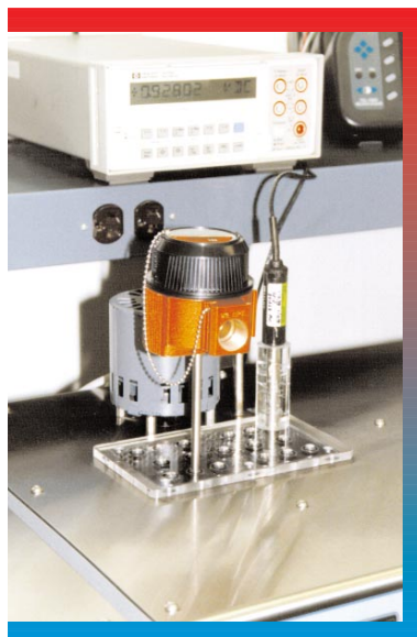
FIG. 1: In transmitter-to-sensor matching, the sensor is immersed in a precise calibration bath at a stabilized temperature and the transmitter is programmed to capture and match the measurement of that individual sensor.
